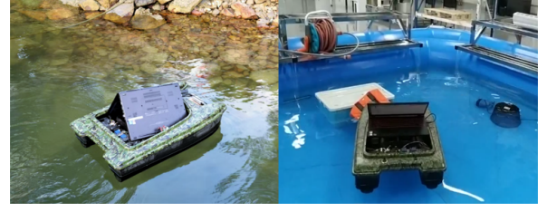
Fig. 8. The USV platform and the working scenarios: nearshore harbor and indoor pool, in the experiments.
