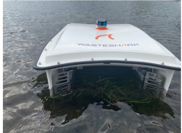
Fig. 1: The WasteShark ASV by RanMarine
