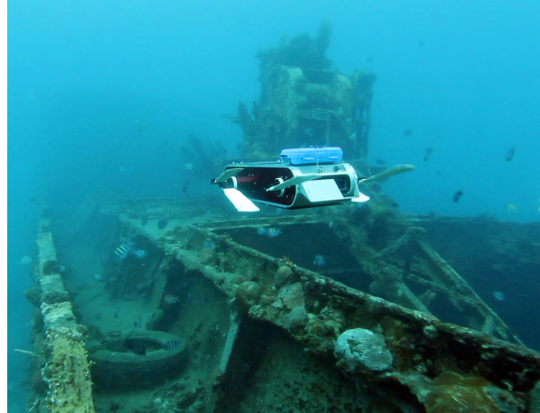
Fig. 1. Aqua2 AUV navigating over the Pamir shipwreck, Barbados.
