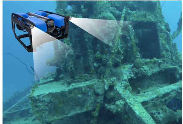
Fig. 1: A photometric stereo framework for non-stationary underwater robots allows low-cost AUVs, like the BlueROV2, here to explore shipwrecks while computing scene reconstruction models, even under dynamic lighting conditions.
